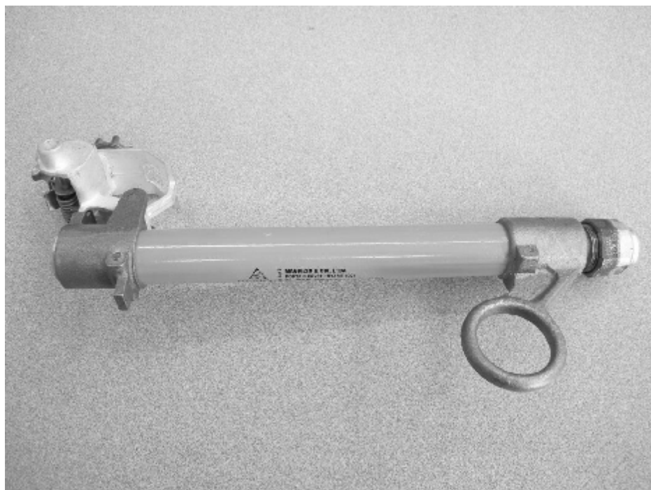
Figure 38. Typical fuse holder used for testing.
