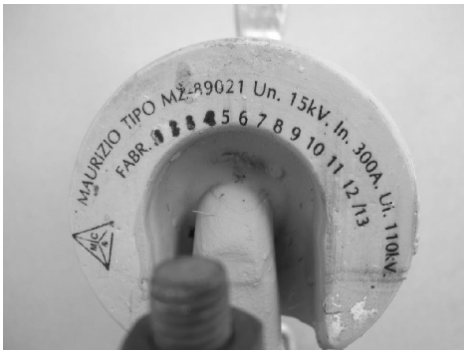
Figure 41. Markings on the insulating support.
