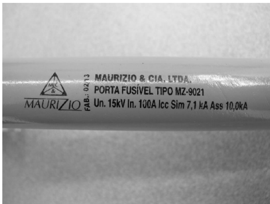
Figure 39. Markings on the fuse holder.
